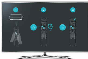
1. Point the remote control at the STB. Do not cover the infrared (IR) window on the front of the remote control or at the front of the STB.
