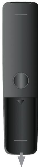
2 Insert 2 x AAA batteries observing the correct polarity
